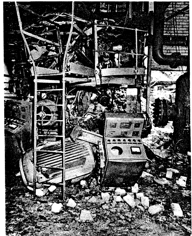
Figure 2. Turbo expanders after explosion.
